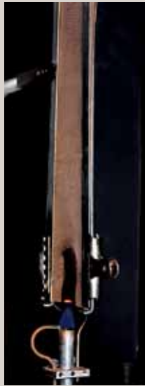
Vertical flame test on UltraSoft® fabric
